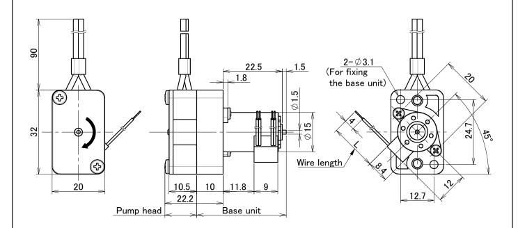
Note: The pump head can be attached to the base unit by rotating the pump head 180 degrees so that the tube is facing downwards.
